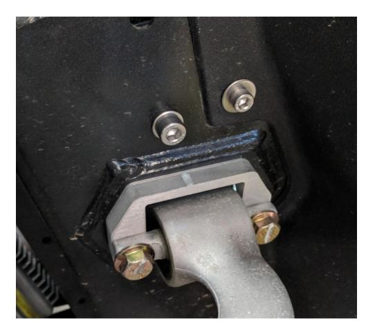
4. Thread M6 flange nut onto the M6 bolt and tighten.
