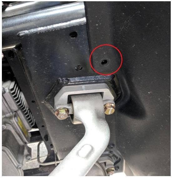
2. Use M6 bolt and washer to replace the bolt removed in the first step. This bolt threads into a nut welded to the chassis. Tighten bolt.
